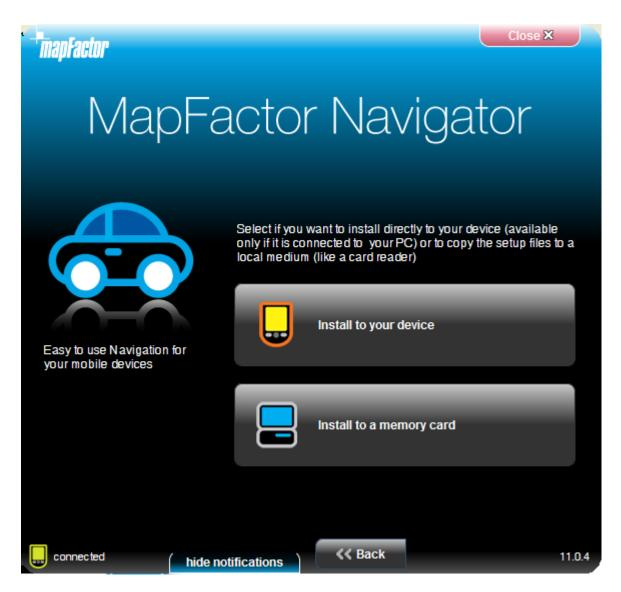
If your device is connected to your PC using ActiveSync or Windows Mobile Centre you can install directly to your device. Otherwise the program or cab file will be copied to an SD card.
