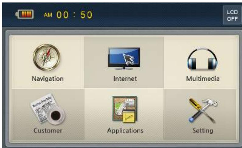
The main menu screen consisted of several icons will appear after switching on the device. All functions can be controlled using the touch screen. In the case that you choose repeatedly to run the application directly after switching on the device, this application will be running on the screen. Multitasking is supported. While you run the navigation, you can listen to music.
